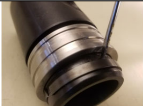
Removal of retaining
